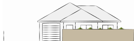
Unsuitable front fencing
