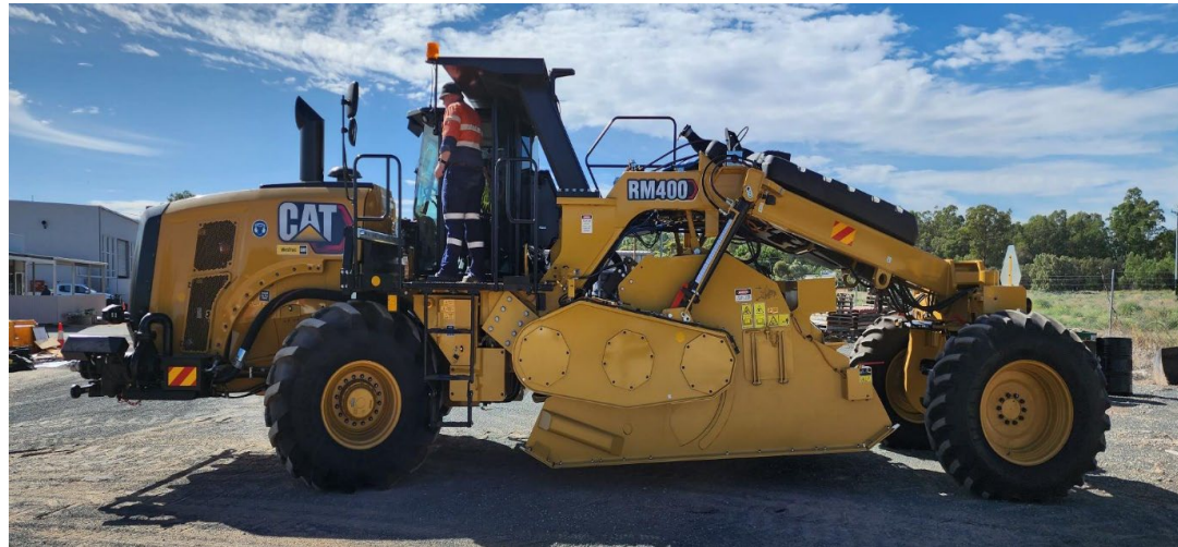
New CATERPILLAR RM400 Road Reclaimer for Barham/Moulamein Works teams.
