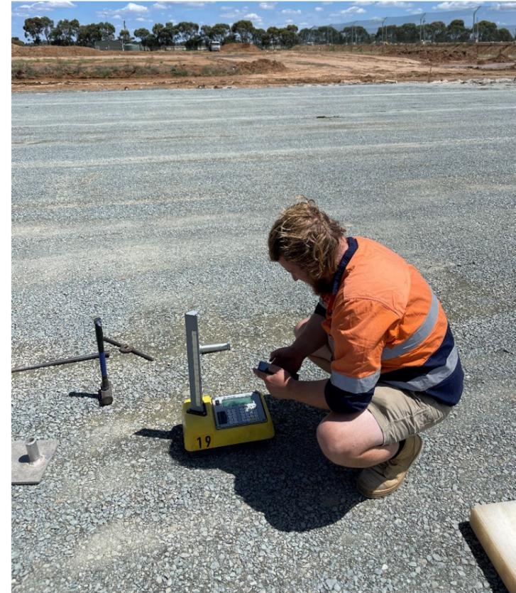
Compaction tests being undertaken on the Automated Depot shed pad.
