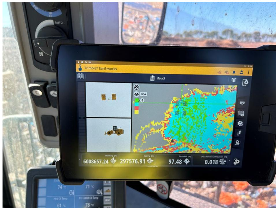
Trimble 3D GPS installed in the CAT landfill compactor showing waste density
