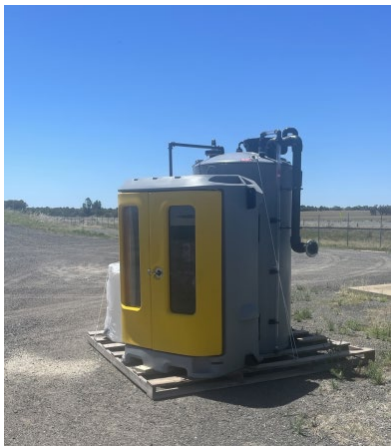
Chemical dosing unit for Wakool WTP
