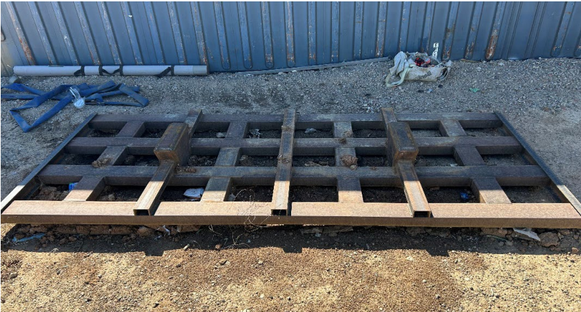
Mark from Engineering fabricated a smudge bar for the new 938 Cat loader to use at Moama Landfill
